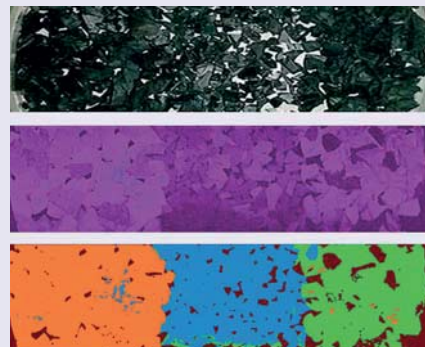
Specimen (photo, top), segment (cutout, section) of hyperspectral measurement at 650 nm (center) and classification (PA6, PA66 and TPU, bottom).
