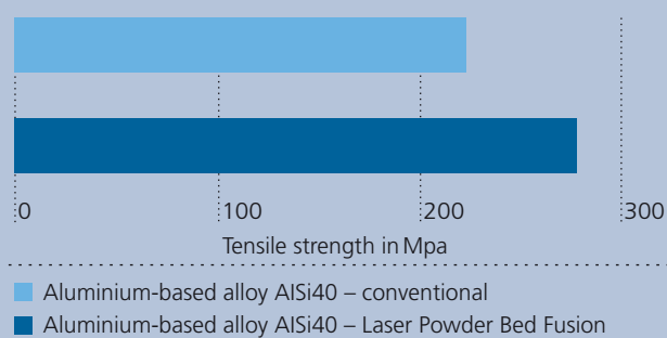
Study of the tensile strength of aluminum-based alloy AlSi40 (60 mass percent aluminum, 40 mass percent silicon)
